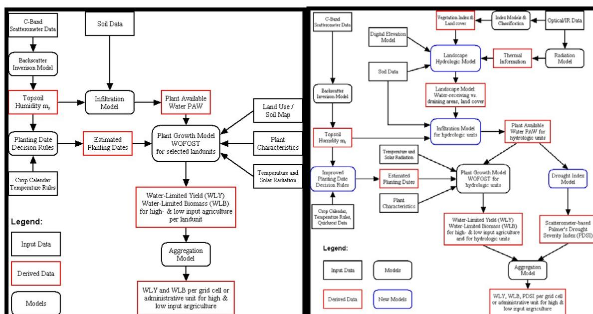
Figure 8-4 Current and future operational methods for DRYMON The new developments to be carried out within this project are indicated by the blue rounded rectangles
