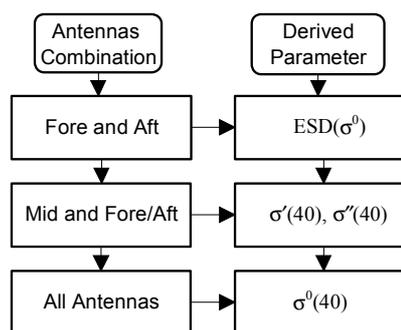
Figure 2-4 Flow chart of processing steps for ERS Scatterometer data. In the processing four parameters are obtained: The estimated standard deviation of  $\sigma^0$ ,  $ESD(\sigma^0)$ , the slope  $\sigma'(40)$  and the curvature  $\sigma''(40)$ , and the backscattering coefficient at 40 degree,  $\sigma^0(40)$ .
