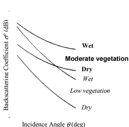
Figure 2-3 Illustration of the dependency of the backscattering function  $\sigma^0(\theta)$  on vegetation and soil state
